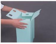
3. Bending the bottom of the box and peel off excess parts then snap the buckle into the hole.
